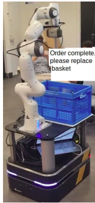
Figure 5.9: Robot returns to its base station and requests a basket change
