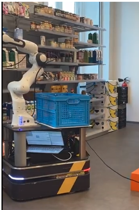
Figure 4.6: The FlexBE behavior in action during the robot simulation (the laptop screen shows the runtime control)
