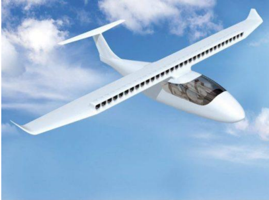
Figure 1 ONERA's Ampere aircraft, which uses distributed electric propulsion.
